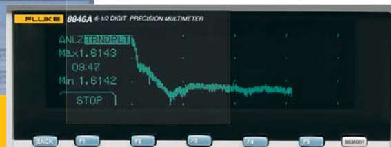
The graphical display on the 8845A/8846A provides context sensitive menus and advanced functions like TrendPlot, histogram and statistics.
