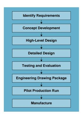
Figure 1 - The Simplified Design Process
